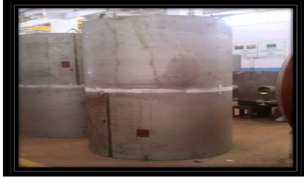
Figure 3. L-seam welding & DP test
